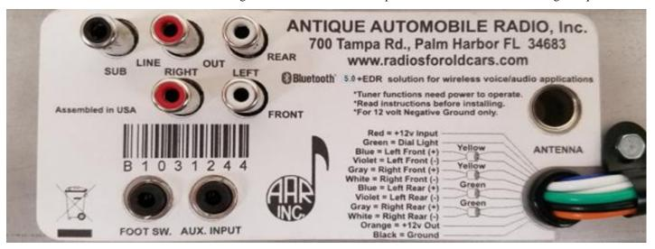
The antenna jack is located above the wiring harness exit. It will accept your original antenna plug.
